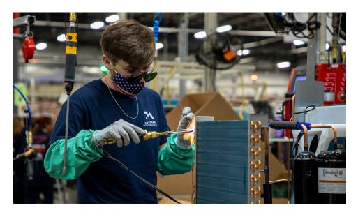
The art of brazing—or using a torch to join two independent pieces of copper or copper and steel when building an air-conditioner or refrigerator—is critical to the overall quality and cooling performance of the unit. At Monogram Refrigeration, craftsmanship is a priority for braze operators who must complete classroom instruction, an apprenticeship consisting of personal coaching and hours of on-the-job training to become fully certified in six months.
